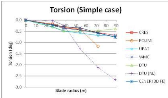
*Prediction of torsional response to simple load case with various numerical models*
