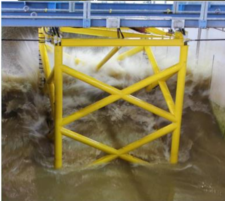
Excerpt of measurement campaigns that have been uploaded: Hybrid testing of a semisubmersible scaled wind turbine (top left), wave slam tests on a jacket-structure
