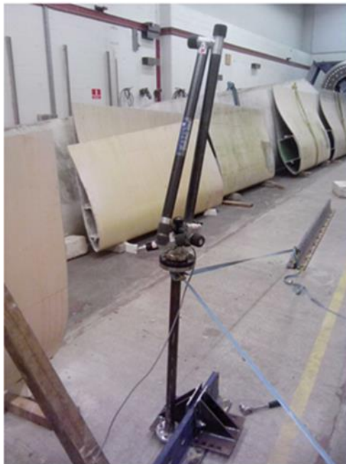
Figure 28: Technical characteristics of FARO ARM and 1m height base.
