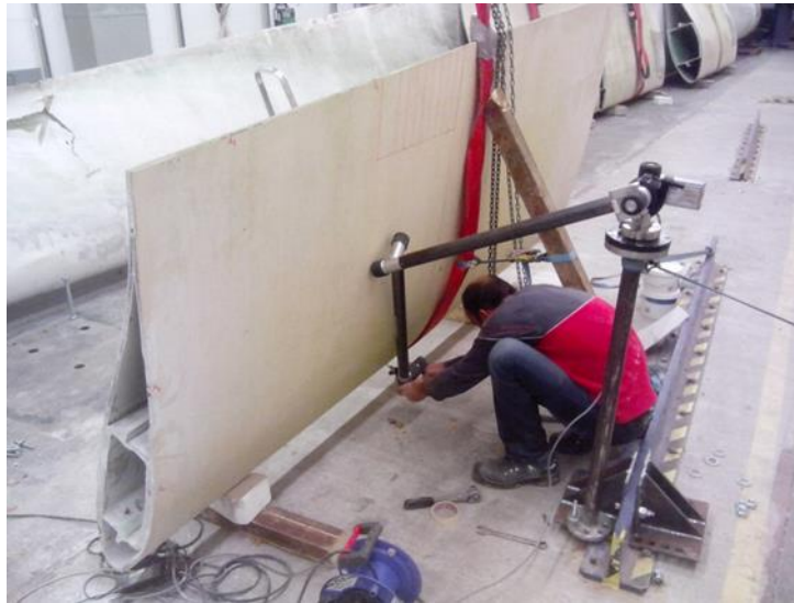
Figure 26: 3D geometry measurements on a 3m sub part in DTU lab.
