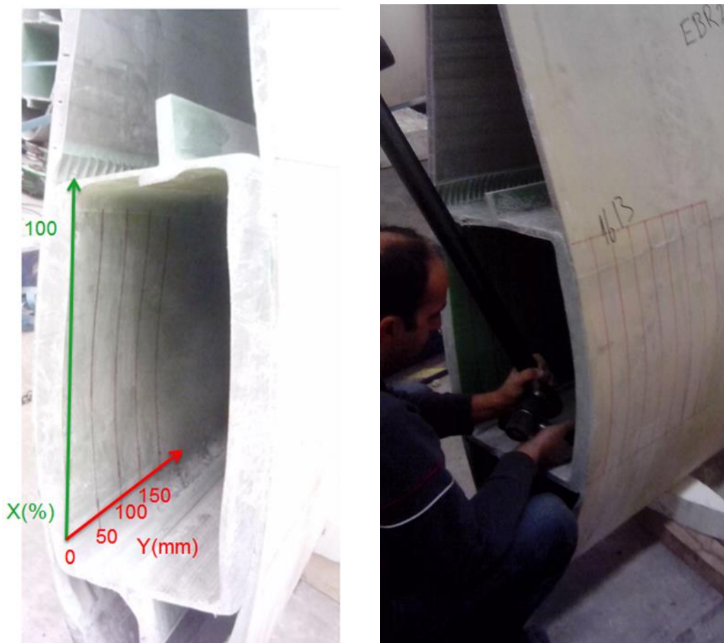
Figure 29: Measuring positions in Y and X direction.
