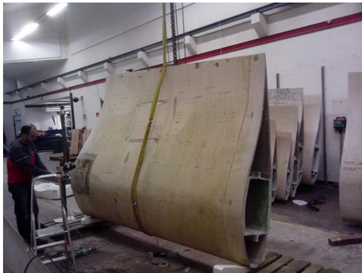
Figure 25: (a) 3D geometry measurements using the robotic arm in DTU by CRES
