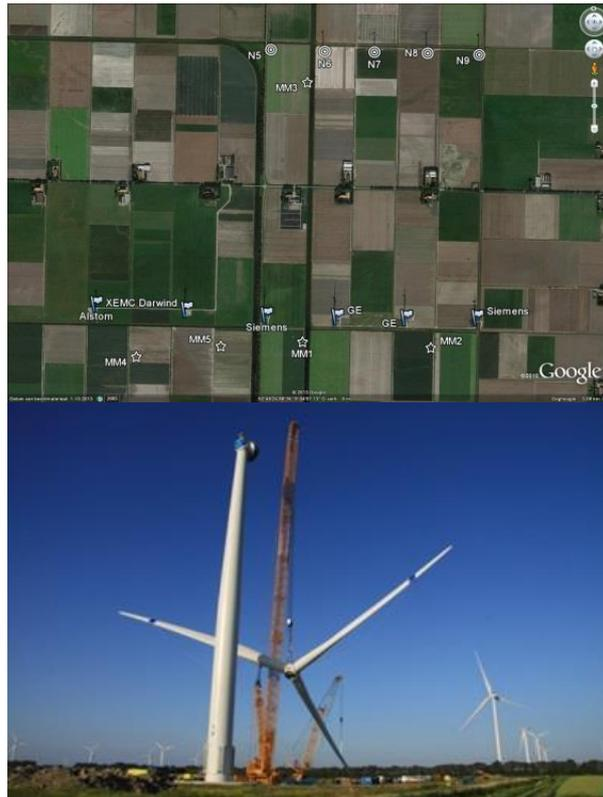
ECN's test site is a unique facility and comprises a combination of a research wind farm, prototype test locations and a remote sensing validation facilities. The site is an onshore site near the lake IJsselmeer and consists of flat, agricultural terrain with single farm houses and rows of trees. The site has a favourable wind climate with an average wind speed of 8,3m/s at 100m height and a mean turbulence level of 8.1%; the main wind
